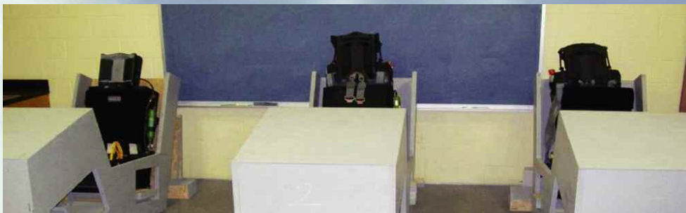
The Seat Comfort Test Bed
