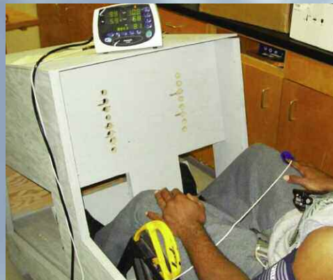
Seat comfort test bed experiment for the sitting mode
