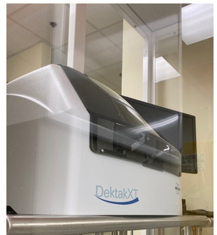
The Nanotechnology Laboratory is the home of a new ridged-walled modular cleanroom. Six new micro and nano fabrication tools were installed, including a Bruker Dektak XT Profilometer.
