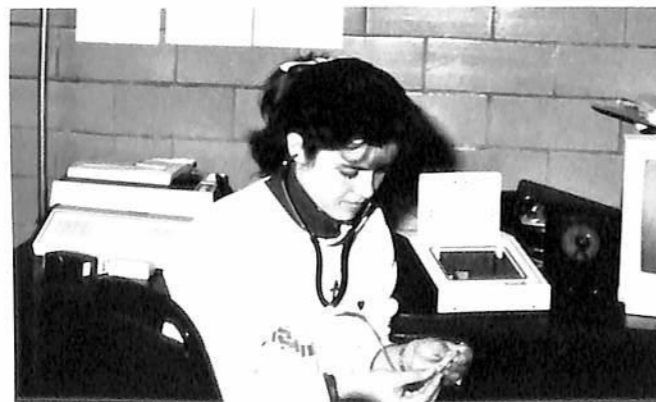
Graduate student, Gretchen Bright, doing a listening check on a hearing aid with a stethoscope.
