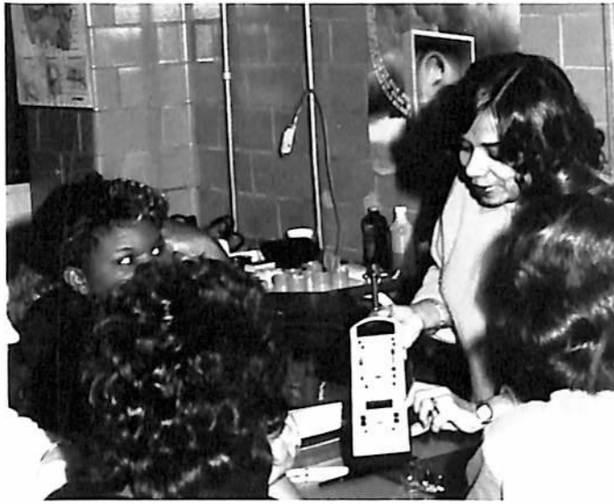
Dr. Zenobia Bagli showing the controls on a sound level meter, used in calibrating and in making noise measurements, to a group of students.
