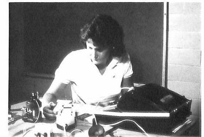
Julia Ninerell, graduate student, calibrating a portable audiometer used in administering hearing screening tests.
