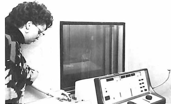
Paulette Dabbs, graduate student, adjusting the recording sheet on an X-Y Plotter, used in automatic hearing tests.
