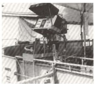
Computer-operated scales provide digital readout and options for automatic drafting, colour branding and recording of data for later use.
