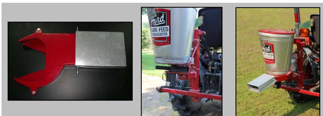
Fig. 5. Left photo: Chute attachment for a Herd® GT-77 spreader. Middle photo: Herd spreader without chute attachment. Right photo: Herd spreader with mounted chute attachment.
