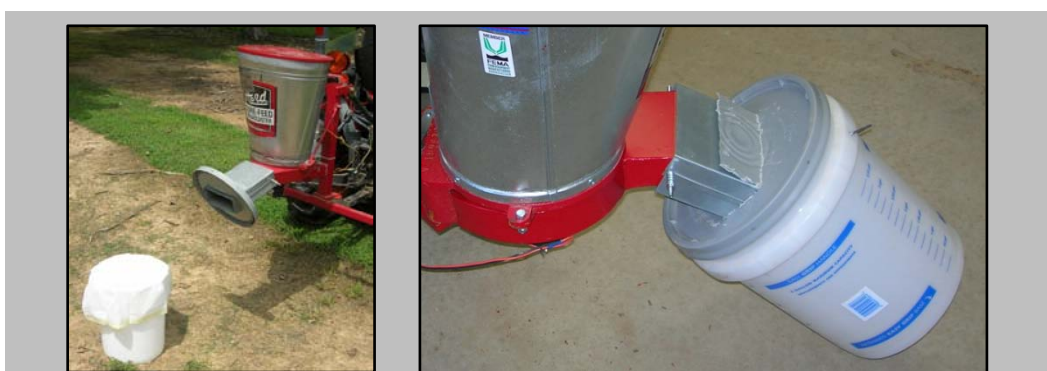
Fig. 6. Left photo: Five gallon bucket lined with trash bag on the ground in front of a Herd® GT-77 spreader with a slotted bucket lid slid over the end of the chute attachment. Right photo: Close-up of bucket lid slid onto chute attachment.
