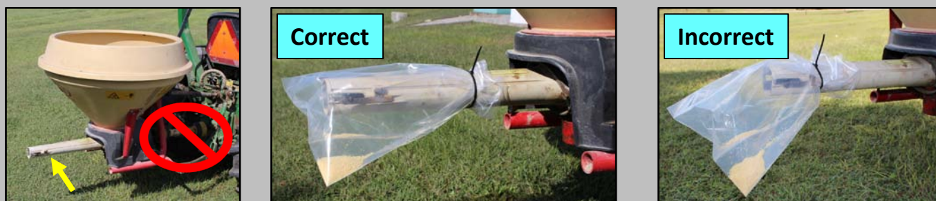
Fig. 7. Left photo: Vicon spreader with detachable spout attachment (see yellow arrow). Do Not go anywhere near the Vicon PTO shaft on the opposite side of the spreader during operation (see red circle with slash). Rotating PTO's Can Be Lethal . Middle photo: Spout attachment with a plastic bag zip-tied to the dispensing spout to catch bait. A bag with thicker plastic (i.e., heavier mil) works best because the moving spout will rub a hole in the bag over time. Note that the plastic bag has been slid onto the spout so that there are only a couple of inches of bag from the end of the spout opening. Do Not go near the swinging spout attachment during operation. Right photo: Plastic bag attached too far back on the spout attachment, which results in bag twisting when the spout is swinging side to side.
