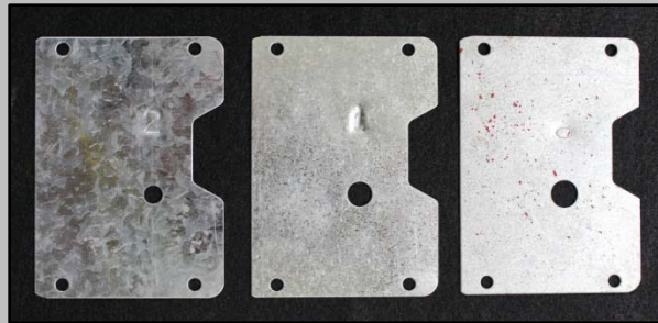
Fig. 1. Herd® spreader blocking plates: #2 ( left image ), #1 ( center image ), and #0 ( right image ). The center hole is where bait drops from the spreader. The four outer holes are used to position the blocking plate on the spreader. The #2 has the smallest diameter hole at 0.28 in (7 mm), followed by the #1 at 0.35 in (9 mm) and the #0 at 0.39 in (10 mm).
