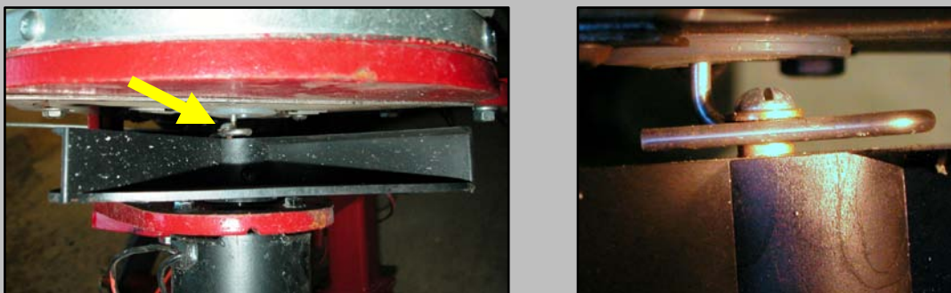
Fig. 2. Left Photo: Area between Herd® spreader hopper and four-bladed fan where stainless steel agitator wire connects to the screw above the fan blades. Right Photo: Close-up image of agitator wire properly positioned with the screw in the middle of the wire hook.
