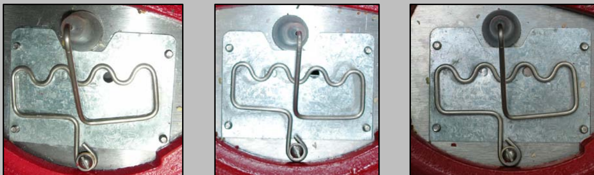
Fig. 3. Left Photo: Blocking plate with gap beneath fully opened. Center Photo: Blocking plate with gap beneath partially closed. Right Photo: Blocking plate with gap beneath fully closed.
