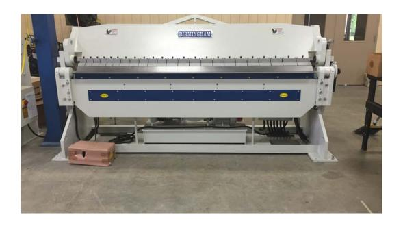
Birmingham 8 ft. x 10 gauge hydraulic metal brake: Machine tool for bending sheet and plate material, most commonly sheet metal.
