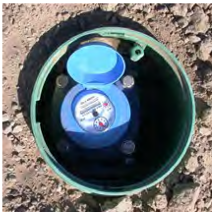
A flow meter measures the water input for strawberry irrigation.
