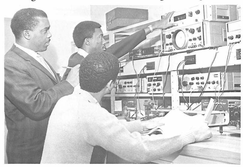
In the Department of Electrical Engineering Wallace R. Perkins supervises these majors as they employ experimental analysis and synthesis of circuits to verify theoretical and mathematical data regarding a linear, time in variant system's response to a specific input.
