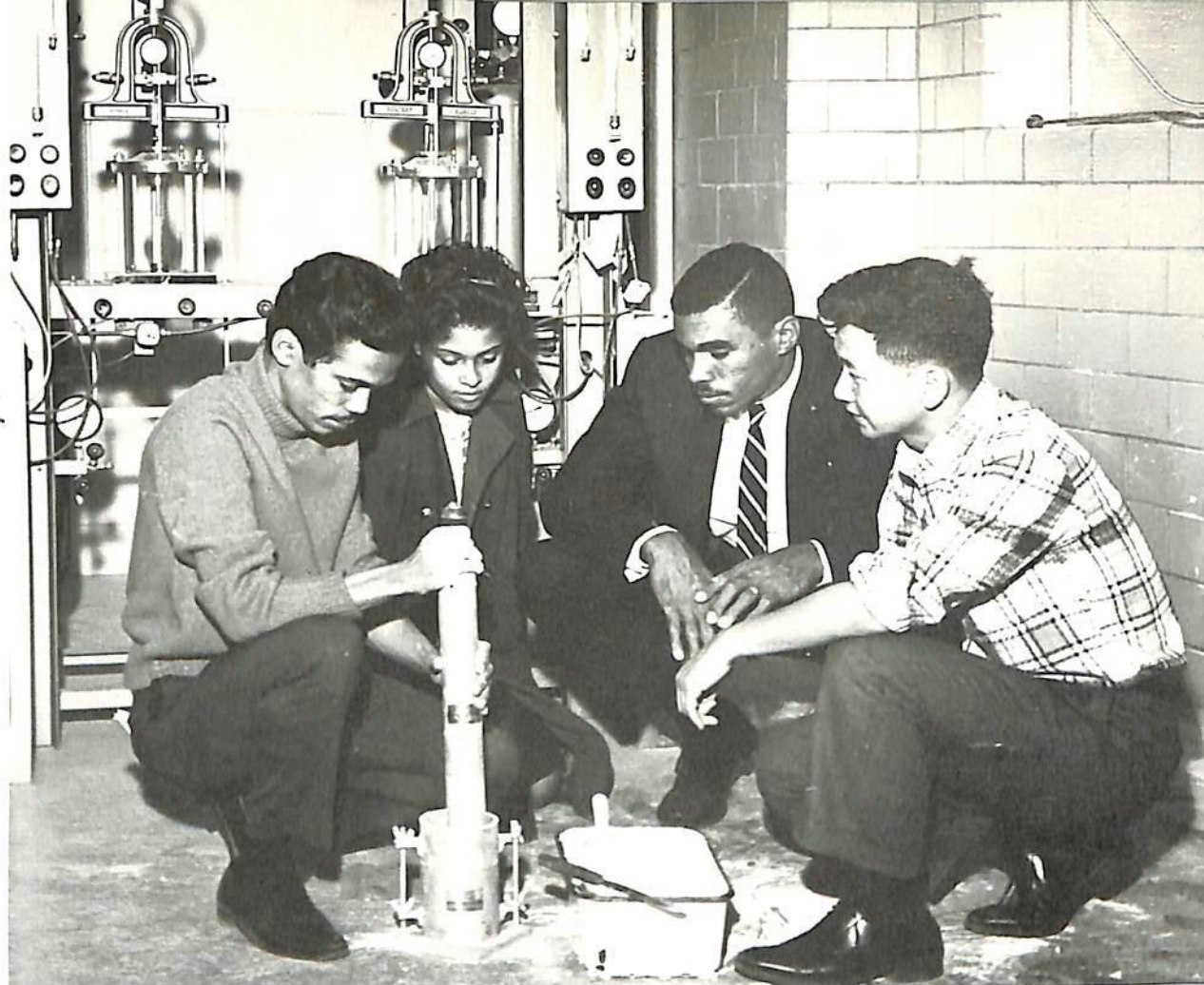
Engineering majors in the soil mechanics laboratory perform compaction to determine maximum dry density and optimum water content that will be used in compacting earth fill for highway or earth dams.
