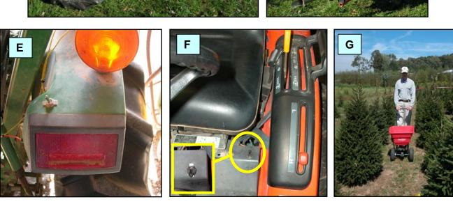
Fig. 1. Images of a tractor-mounted (A and B) Herd spreader or (C and D) Vicon spreader; an on / off switch for the Herd spreader mounted on the (E) fender of a tractor or (F) beneath the tractor seat; and (G) an Earth-Way push spreader being used to apply fire ant bait in a commercial nursery.
