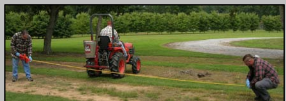
Fig. 4. Measure the bait spreader swath width.
