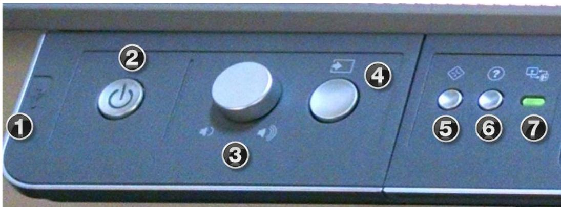
1. **USB Port** – Most Master Controller Trays contain a USB port
