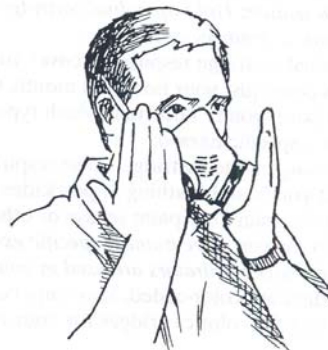
Negative pressure test
