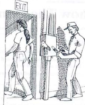
Unauthorized workers should leave the area before cleaning or repairs begin.
