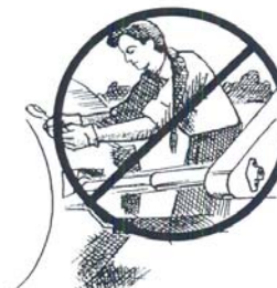
Tie back and tuck in long hair when working near a PTO shaft.
